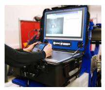
SERVICAM's: Portable weld **monitoring** and **supervision** system.
