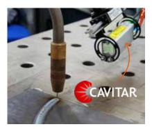
Cavitar's revolutionary welding camera uses laser illumination to see through the welding arc.
