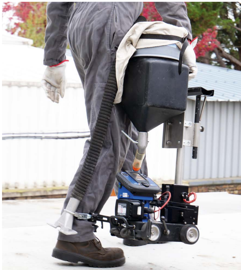
Kit AS sur un chariot de soudage GLUMAG® EVO
